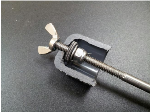
Note rubber washer under cap needed to seal
