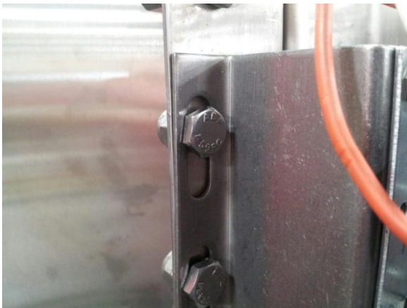
Base is adjusted up or down for correct chain length
