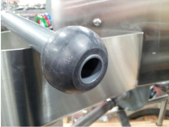
Inspect drain ball for grooves or lumps that cause leaks
