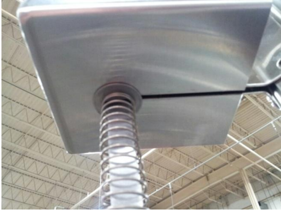
Large washer goes on outside of solenoid cover
