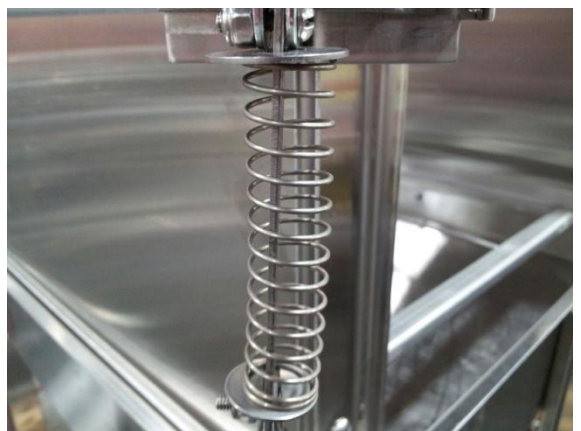
Large washer 086-6607 on top, small 086-6606 bottom
