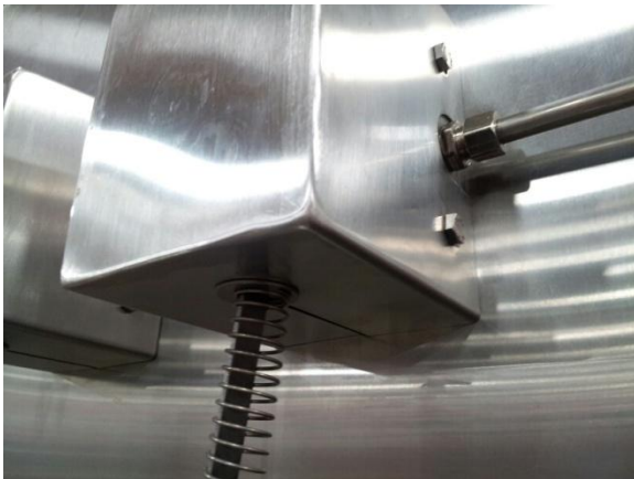
Solenoid cover on 5AG-S, dual solenoids
