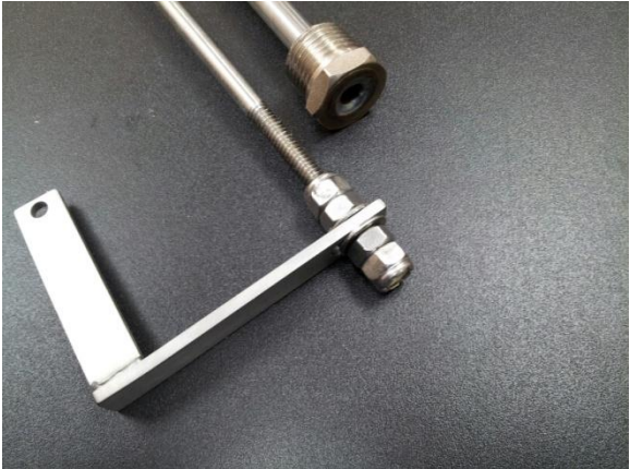
Link 085-6610 secured to pushrod, no packing in tube
